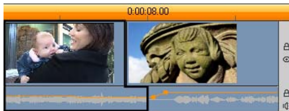
Audio cuts after video. The resulting “L” shape is outlined in this illustration.
