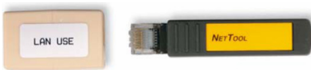
Figure 3. Cable Coupler and Cable Identifier
