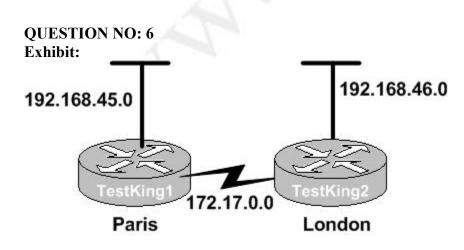
A network administrator in London has been instructed to prevent all traffic originating on the Paris LAN from entering the TestKing2 router.
