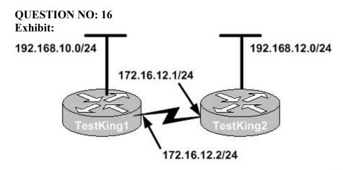
The network administrator of the TestKing1 router adds the following command to the router configuration: ip route 192.168.12.0 255.255.0 172.16.12.1 What are the results of adding this command? (Choose two)
