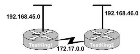
A network administrator has been instructed to prevent all traffic originating on the TestKing1 LAN from entering the TestKing2 router.
