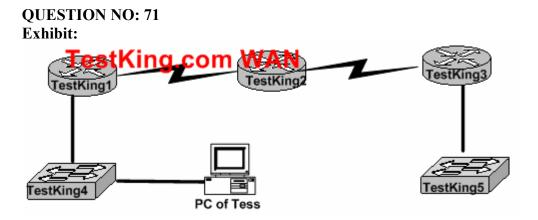
An employee Tess of TestKing company has moved to an office on a different floor. Although the administrator is able to telnet to all of the routers, the address of Switch TestKing5 is needed in order to verify that Tess remains in the same VLAN.
