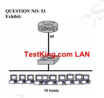
Refer to the topology shown in the graphic. Each host is connected through its own 10Mbps half-duplex switch port to the e0 interface of the router TestKing1. What is the bandwidth available to each host?
