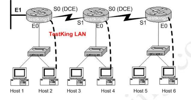
Task: To configure the router click on a host icon that is connected to a router by a serial console cable.
