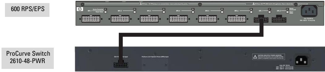
Figure 4-4. Example of an 600 RPS/EPS Powering One 2610-48-PWR Switch
