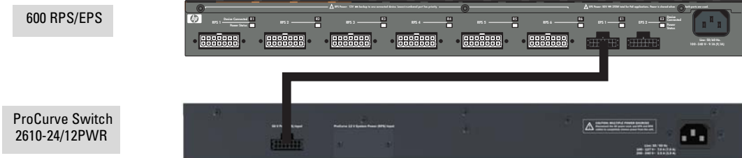
Figure 4-1. Example of a 600 RPS/EPS Powering One 2610-24/12PWR Switch
