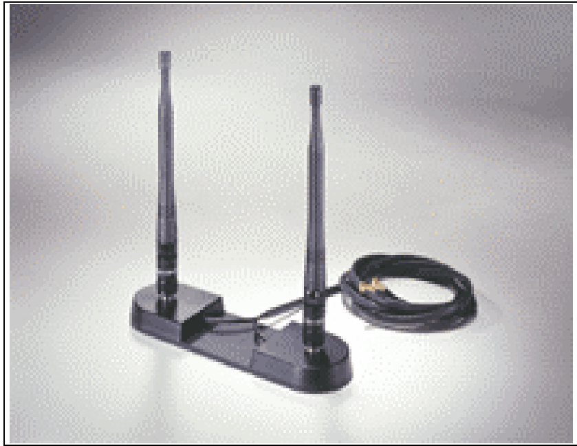
Figure [10]: A double dipole antenna
