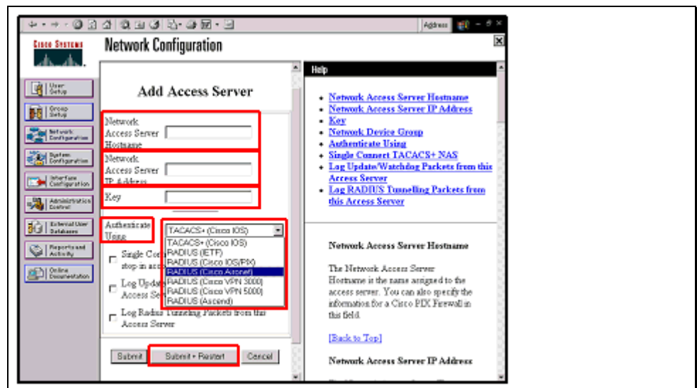
Figure [3]: Access Server Setup Example
