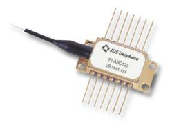
The JDS Uniphase 2900 Series 980 nm pump module utilizes a planar construction with chip on subcarrier. The high power JDS Uniphase laser chip is hermetically sealed in a low-profile, epoxy- and flux-free 14-pin butterfly package and fitted with a thermistor, thermoelectric cooler, and monitor diode. This product uses a polarization maintaining fiber (PMF) pigtail that allows excellent side mode supression ratios (SMSR) over a very wide dynamic range.
